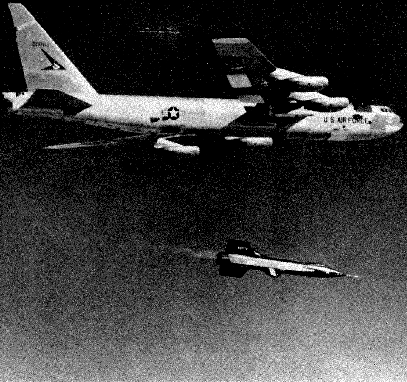
Shown seconds after release from its Boeing B-52 mother ship is the USAF X-15 research vehicle, which has been designed to probe the fringes of space. Le X15 se détache de l'avion transporteur.
